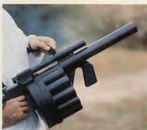
LEFT: Developed decades ago as riot-control weapon, 40mm grenade launcher is reborn as MM-1, firing 12 of any mix from smoke, gas, beehive or HE ammo sefection. Inserts for 12-ga. are available for 16-lb. revolver.
